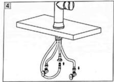
Connect hot and cold water supply lines to the Water Supply Valves.
