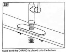
Make sure the O-RING is placed onto the obtain of Base Ring. Install faucet through Deck Plate. From underside sink, put Plastic Washer and Mounting Nut. Position faucet on sink properly and tighten Mounting Nut.
