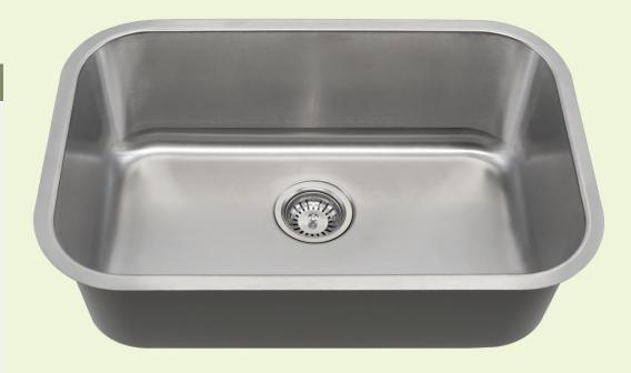
27 1/8" x 17 7/8" x 9 3/8" Undermount Installation 30" Minimum Cabinet Size 16- or 18-Gauge Steel Available Certified High-Quality 304 Stainless Steel Brushed Satin Finish Offset Drain Thick Sound Dampener Rubber Pad Fully Insulated Cardboard Cutout Template Included Installation Hardware Included Limited Lifetime Warranty
