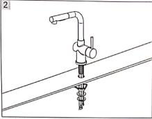
Install without Deck Plate. Make sure the O-RING is placed onto the bottom of Base Ring. Install faucet through hole in sink. From underside sink, put Plastic Washer and Mounting Nut. Position faucet on sink properly and lighten Mounting Nut.
