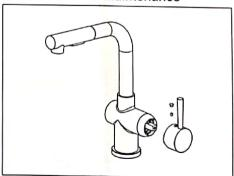
Turn off water and reliev a pressure! Detach handle button using a small flathead screwdriver, unscrew set screw using Allen Wrench and take off handle.
