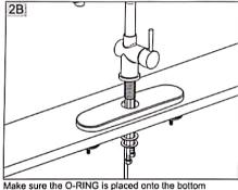
Make sure the O-RING is placed onto the bottor of Base Ring. Install faucet through Deck Plate. From underside sink, put Plastic Washer and Mounting Nut. Position faucet on sink properly and tighten Mounting Nut.
