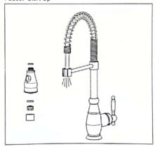
After installation is complete, remove aerator and rotate handle to the closed position. Turn on the water supply valves, and check all connections for a leak. Turn on your faucet and allow both hot and cold water to run at least one minute each. Replace Aerator.
