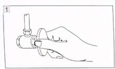
Remove any debris from valve outlets. Turning off the water supply valves. This is usually found near the water meter. If you are replacing an existing faucet, remove the faucet from the sink and clean the sink surface thoroughly.
