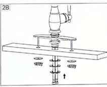
Install with deck plate. Assemble mounting screws onto underside of deck plate. Position deck plate onto 3-hole mount of sink. From underside of sink, tighten plastic mounting nut. Make sure the O-RING is placed onto the bottom of Base Ring of faucet. Install faucet through hole in deck plate. From underside of sink, attach mounting assembly. Position faucet on deck plate properly and tighten Mounting Nut.
