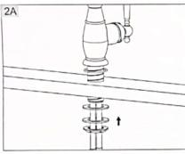
Install without Deck Plate. Make sure the O-RING is placed onto the bottom of Base Ring. Install faucet through hole in sink. From underside sink, attach mounting assembly Position faucet on sink properly and tighten Mounting Nut.
