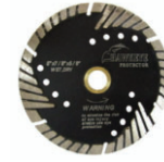
Hawkeye Protector Turbo Granite Blade with Side Protection Size: 5", 6", 7" Cuts Wet/Dry: Granite, Quartz, Quartzite
