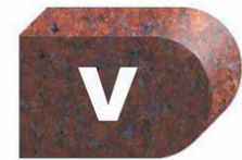
Full Bullnose Profiling Bit Size: 2cm, 3cm, 4cm, 5cm, 6cm (5cm & 6cm - special order)
