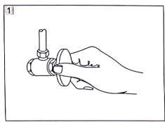
You should clean all the dirts from valve outlets. Turning off the water supply valves. This is usually found near the water meter. If you are replacing an existing faucet, remove the faucet from the sink and clean the sink surface thoroughly.
