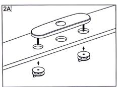
Install with Deck Plate. Place a bead of plumber's putly between faucet and sink. Place Deck Plate over the three holes of sink. From underside sink, tighten Wing nut.
