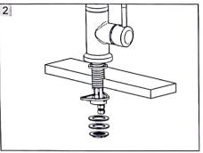
Install without Deck Plate. Make sure the O-RING is placed onto the bottom of Base Ring. Install faucet through hole in sink. From underside sink, put Plastic Washer and Mounting Nut. Position faucet on sink properly and lighten Mounting Nut.
