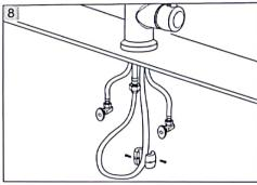
Attach Weights to the pull-out hose using screws at the proper point of the hose. Be noted Weights are optional.
