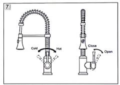
Lift the handle up, the cartridge will be activated allowing water to flow. The water flow will increase by continuing to rotate handle. By rotating the handle to the right, the water temperature will decrease to cold flow only. By rotating Handle to the left, the water temperature will increase to hot only.
