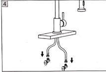
Connect hot and cold water supply lines to the Water Supply Valves.
