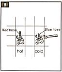
Clean and connect them to the water supplying valve(left to hot water and right to cold.
