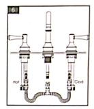
Connect the flexible hoses to the valve bodies. Left hose is for hot water and right for cold.
