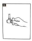
You should clean all the dirts. Turn off the water supply valves. This is usually found near the water meter. If you are replacing an existing faucet, remove the faucet from the sink and clean the sink surface throughly.
