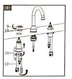
Put the locknut(9),O-ring(10) on the valve body(12) successively. Put the valve body (12) through the Ø28mm hole from under. And tight the locknut(9).
