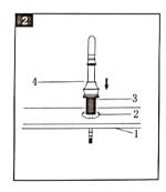
Drill a@33-@35mm hole (2) in sink (1). Install the screw (3) into the faucet body (4). And screw them firmly, insert the them through the hole(2).
