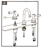
Lock the handle (13) on the valve bodies firmly.
