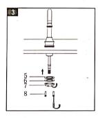
Put all hose through the plastic gasket (5) then through metal gasket (6), finally screw the fitting nut (7), tight it with screw(8).
