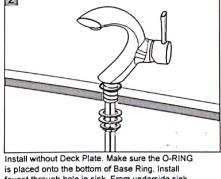
faucet through hole in sink. From underside sink, put Plastic Washer and Mounting Nut. Position faucet on sink properly and tighten Mounting Nut.
