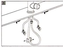
Attach Weights to the pull-out hose using screws at the proper point of the hose. Be noted Weights are optional.
