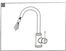
After installation is complete, remove Spray head and rotate handle to the close position. Turn Water Supply Valves on, and check all connections for leak. Flush faucet by running hot and cold water in full position for one minute.
