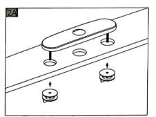
Install with Deck Plate. Place a bead of plumber's putty between faucet and sink. Place Deck Plate over the three holes of sink. From underside sink, tighten Wing nut.
