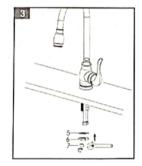
Put all hose through the C Rubber washer (5) then through the C metal Washer (6), finally screw the nut fitting (7).
