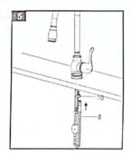
Connect the hose (8) with outlet pipe (10).
