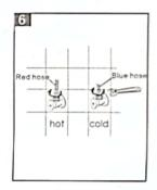
Check the flexible hoses to make it clean and connect them to the water-supplying value(left to hot water and right to cold)
