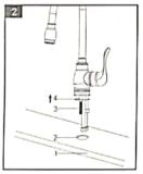
Drill a Ø1-3/8" to Ø1-1/2 hole (2) in sink (1). Install the thread tube (3) and screw them firmly. Put O-ring (4) into base groove and then insert the them through the hole (2).
