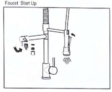
After installation is complete, remove aerator and rotate handle to the closed position. Turn on the water supply valves, and check all connections for a leak. Turn on your faucet and allow both hot and cold water to run at least one minute each. Replace Aerator.
