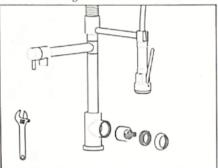
Remove handles. Unscrew Dome Cap counter clockwise by hand. Unscrew Retaining Nut using adjustable wrench, take out cartridge assembly and inspect. Replace parts as necessary. Reassemble parts by reversing steps.
