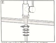
Install without Deck Plate. Make sure the O-RING is placed onto the bottom of Base Ring. Install faucet through hole in sink, From underside sink, put Plastic Washer and Mounting Nut. Position faucet on sink properly and tighten Mounting Nut.
