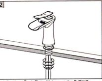
Install without Deck Plate. Make sure the O-RING is placed onto the bottom of Base Ring, Install faucet through hole in sink. From underside sink, put Plastic Washer and Mounting Nut. Position faucet on sink properly and tighten Mounting Nut.
